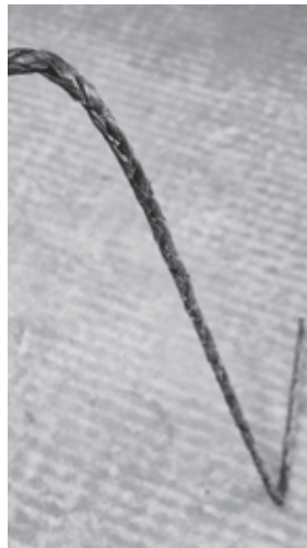
Fig.1: CFRP shaped braided yarn made by Johne & Groß GmbH
